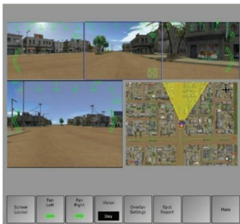
Fig. 1 Vehicle Commander (VC) Warfighter-Machine Interface (WMI), consisting of a 180o field-of-view banner across the top, a 60o field-of-view window on the left hand side, and an overhead map on the right hand side. www.researchgate.net
