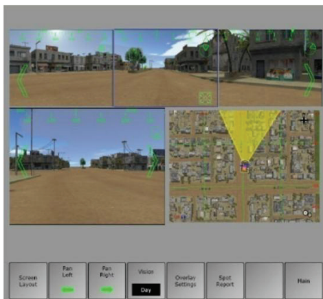
Fig. 1 Vehicle Commander (VC) Warfighter-Machine Interface (WMI), consisting of a 180o field-of-view banner across the top, a 60o field-of-view window on the left hand side, and an overhead map on the right hand side. www.researchgate.net
